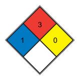
HEALTH 1 Exposure would cause irritation with only minor residual injury (e.g. <u>acetone</u>, sodium bromate, potassium chloride)
