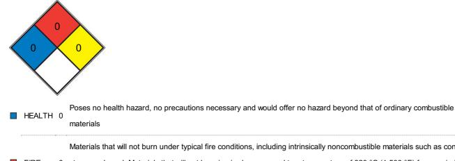
Materials that will not burn under typical fire conditions, including intrinsically noncombustible materials such as concrete,
